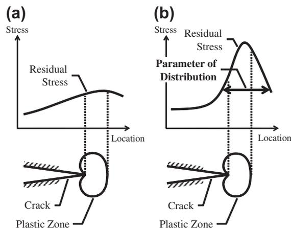
**Fig. 1.** Schematic diagram showing the positional relationship between the plastic zone and the residual stress distribution for: (a) the gentle distribution of the residual stress and (b) the steep distribution of the residual stress.
