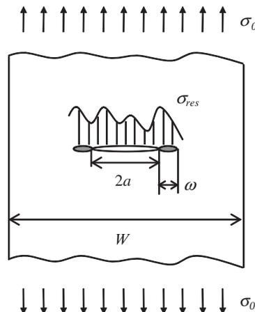
Fig. 2. Center crack tension specimen with residual stress and plastic zone.
