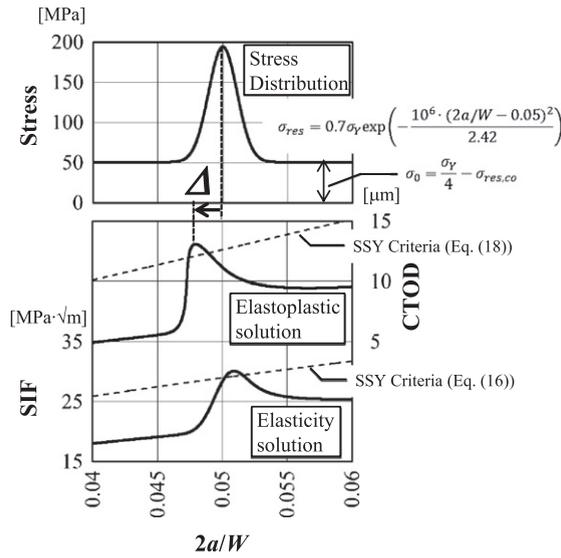
Fig. 4. Example of analytical results for: upper, stress distribution ( $=\sigma_0 + \sigma_{res}$ ); middle, analytical results of CTOD as the elastoplastic solution; lower, analytical results of SIF as the elasticity solution.
