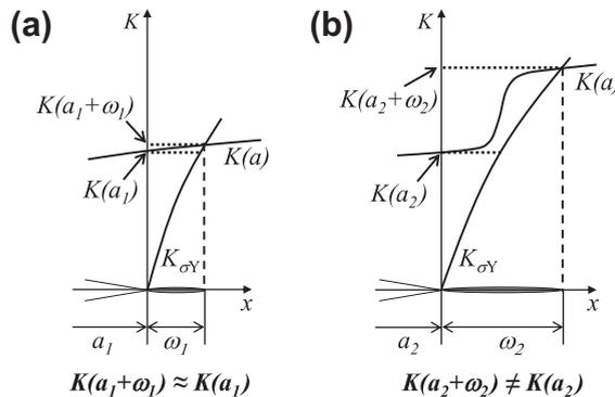
Fig. 8. Schematic diagram showing the relationship between the SIF function and plastic zone size in the Dugdale model for: (a) a low-slope SIF and (b) a steep-slope SIF.
