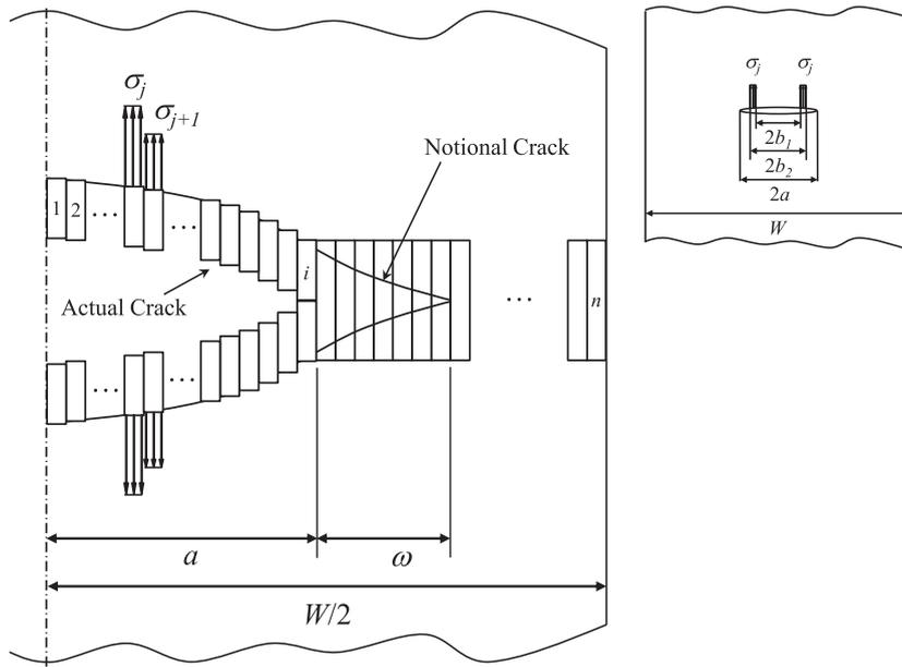
Fig. 3. Schematic diagram of Newman's model.
