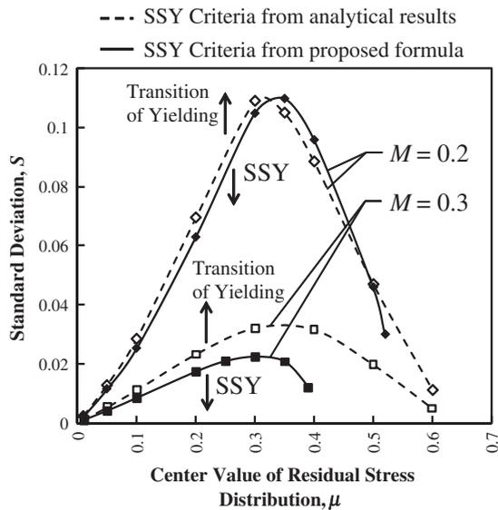
Fig. 9. SSY criteria according to Eq. (26), the formula used with residual stress. Dashed lines show the analytical results presented in Fig. 5.
