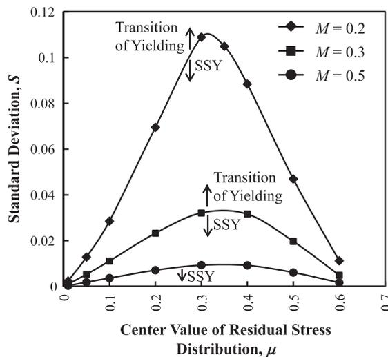
Fig. 5. Analytical results of the SSY criterion for different parameters of the normal distribution  $\mu$ ,  $S$ , and  $M$ .
