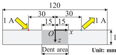
Fig. 3. Schematic representation of the analysis model of the laminate with dents with the area  $-15 \text{ mm} \leq x \leq 15 \text{ mm}$  throughout the thickness.
