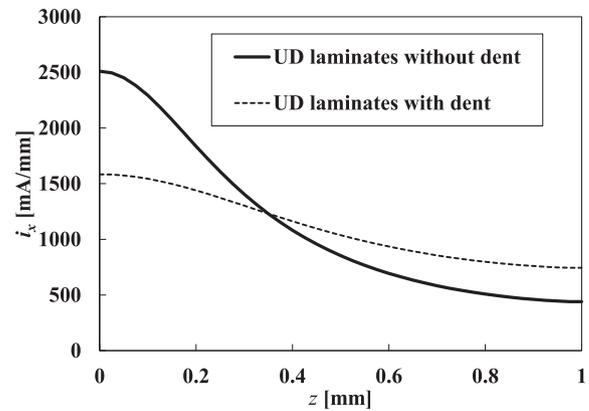
Fig. 8. Comparison of electric current density distributions between beams without a dent and with a dent.
