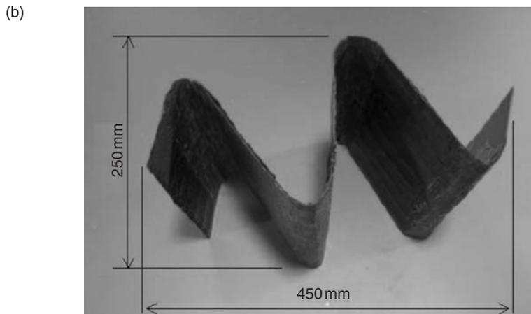
**Figure 18. Self-deployment structure model: (a) Configurations of specimen and (b) Folded type.**
