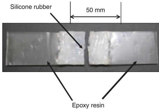
Figure 4. Resin bonding test specimen after tensile test.
