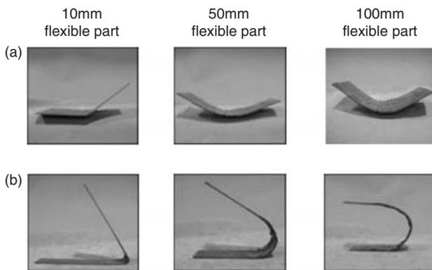
**Figure 13.** Folded specimen configurations at completely unloaded condition of various dimensions: (a) Width of specimen = 80 mm and (b) Width of specimen = 20 mm.
