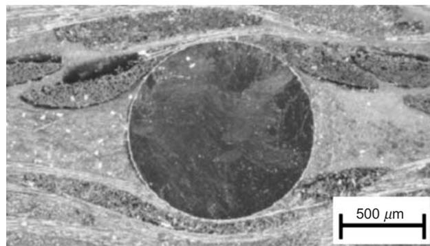
**Figure 15.** Cross section of SMA wire after the first bending.
