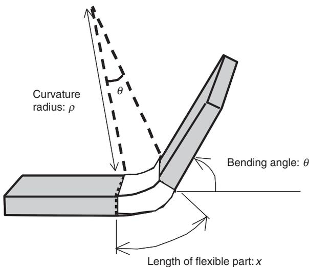
**Figure 9.** Definition of bending curvature radius.
