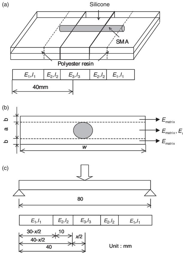
**Figure 16.** Equivalent bending elastic modulus model: (a) Specimen model, (b) Bending elastic modulus model, and (c) Configuration of 3-point bending test.
