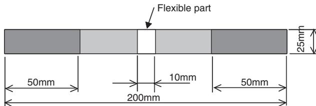
Figure 5. Tensile test specimen of PFC.
