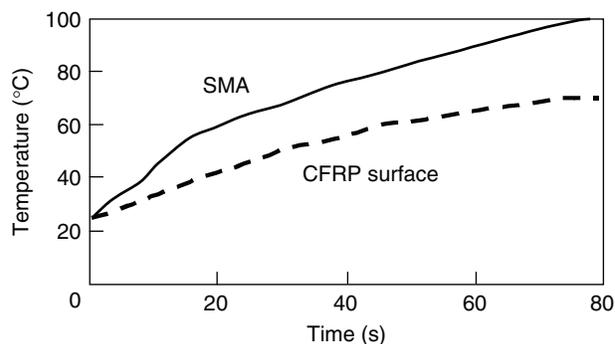
**Figure 20.** Temperature change due to Joule heating.
