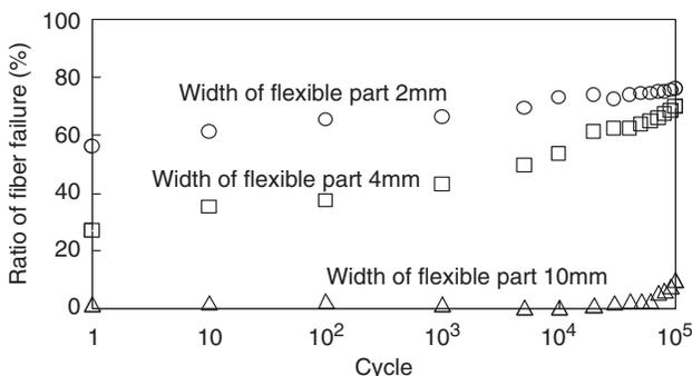
Figure 11. Results of cyclic bending test.
