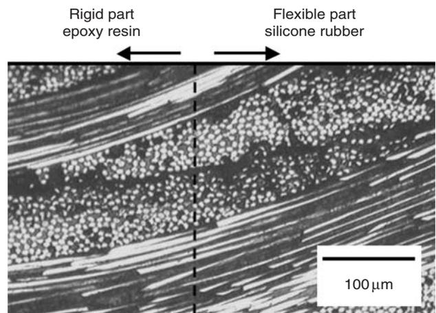
**Figure 3.** Cross section of flexible folding line.
