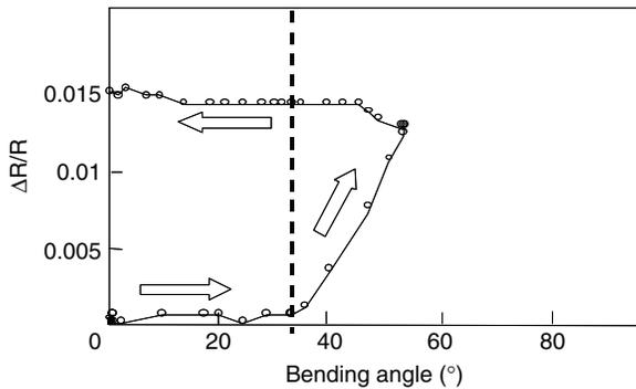
**Figure 8.** Electrical resistance change during bending of specimen with 2 mm flexible length.
