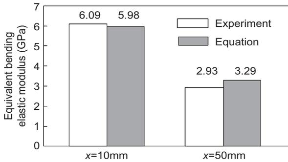
**Figure 17. Comparison of experiment and analytic equation in partially flexible CFRP with SMA embedded.**
