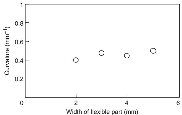
**Figure 10.** Measured fiber breakage curvature of various flexible part lengths.
