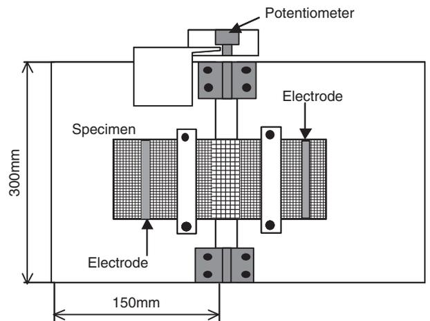
Figure 7. Bending apparatus for PFC with electrical resistance change method.
