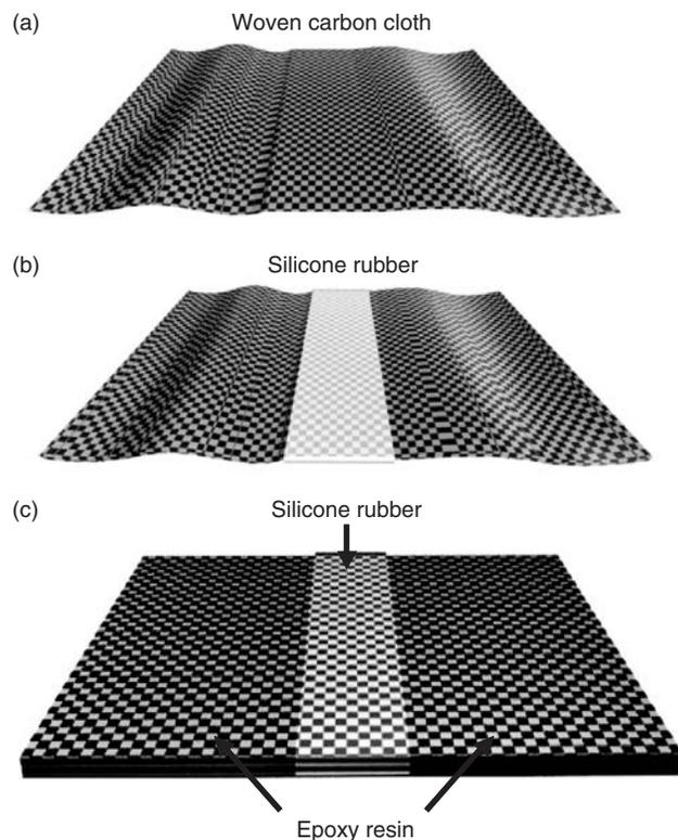
**Figure 1.** Fabrication process of partially flexible composites: (a) Woven carbon cloth, (b) Painting of silicone rubber, and (c) Epoxy resin impregnation.
