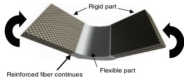
**Figure 2.** Bending of partially flexible composites.
