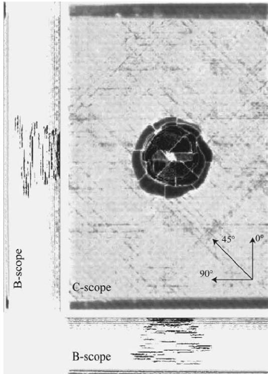
Fig. 12. Ultrasonic testing result of drop weight impact test (6.7 J/mm).
