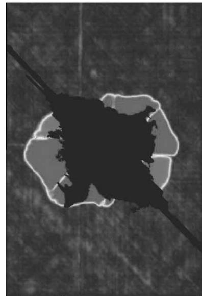
Fig. 11. The overlaid image of UT scanning and the resins deterioration area.
