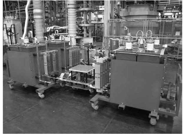
Fig. 2. Impulse current generator (ICG): produced by Nisshin Electric Co.
