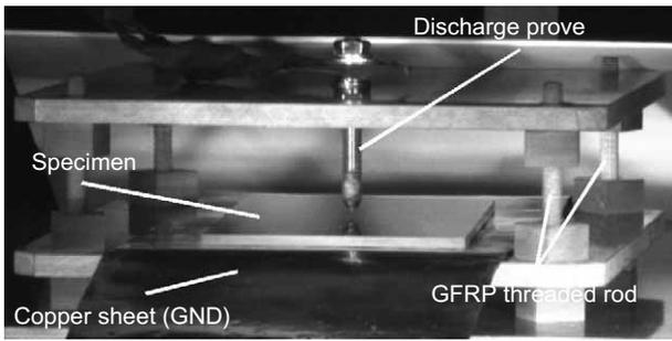
(a) Support jig and specimen setup
