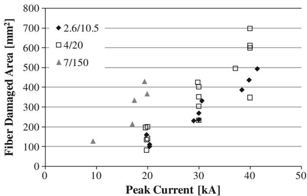
**Fig. 19.** Relationship between fiber damaged area and peak current.
