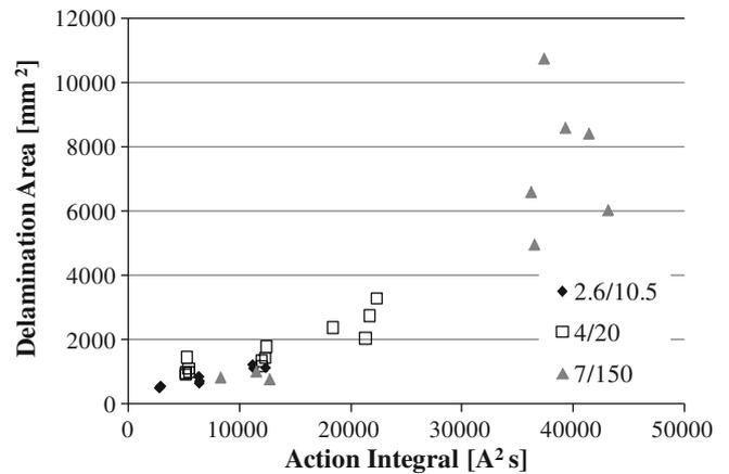
**Fig. 22.** Relationship between action integral and delamination area.
