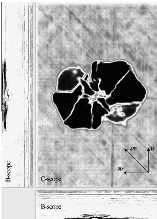
Fig. 10. Ultrasonic testing result of artificial lightning test.
