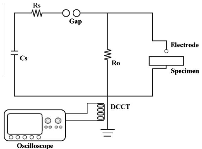
Fig. 3. Illustration of circuit for the impulse testing machine.
