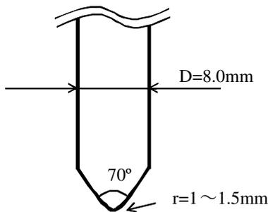
(b) schematic of discharge plove and dimensions
