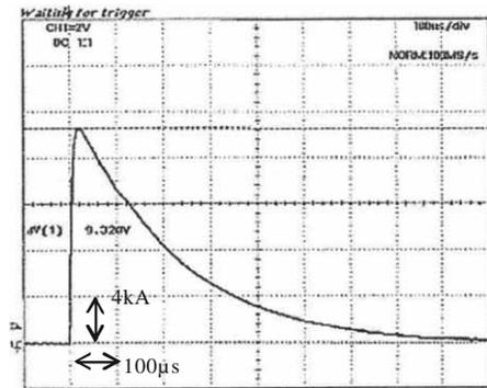
(b) tested waveform with ICG (condition VII)
