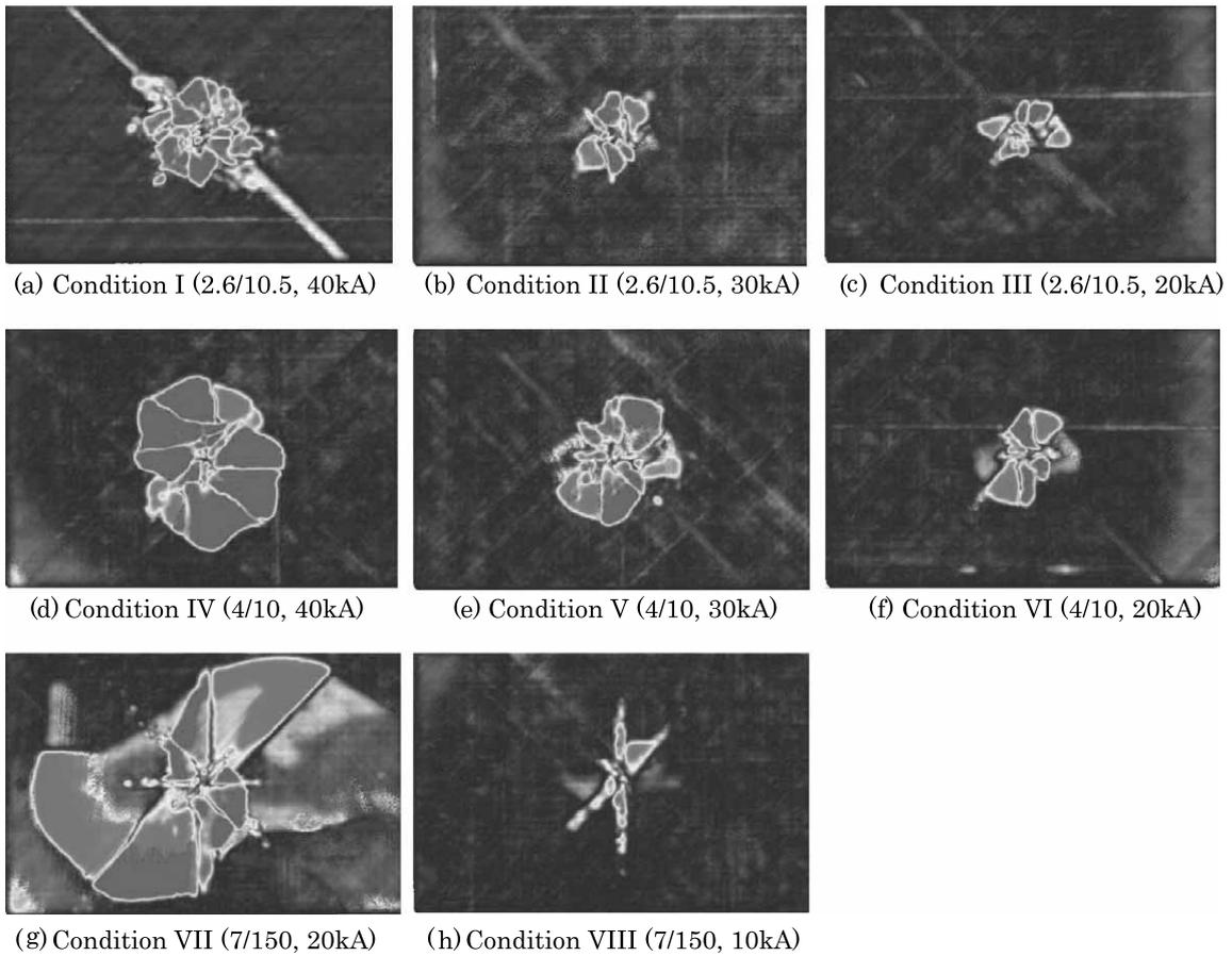
Fig. 9. C-scan image of post-lightning specimen.
