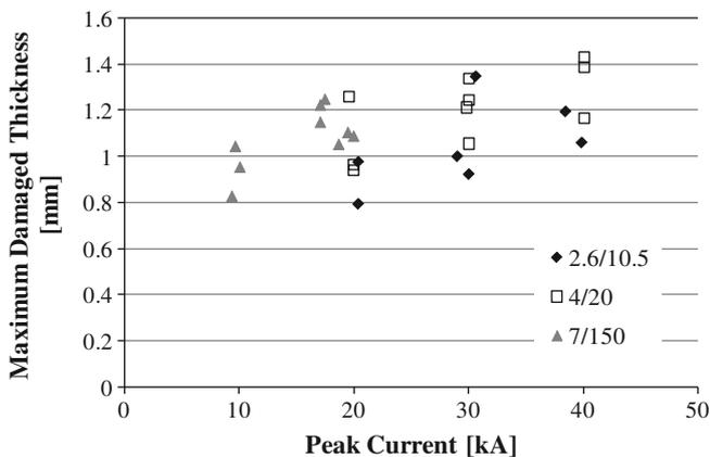
**Fig. 20.** Relationship between maximum damaged depth and peak current.
