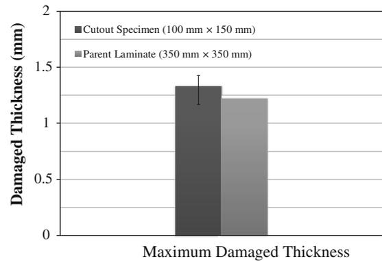
**Fig. 18.** Comparison of maximum damaged thickness between small specimens and parent laminate (condition IV: 4/20  $\mu$ s, 40 kA).
