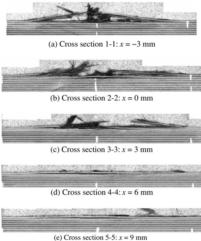
Fig. 13. Sectional observation results (condition IV: 4/20  $\mu$ s, 40 kA,  $t = 4.7$  mm).
