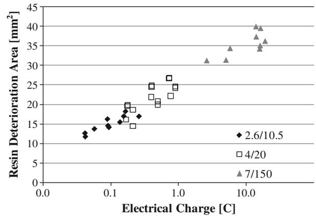
**Fig. 21.** Relationship between electrical charge and resin deterioration area.
