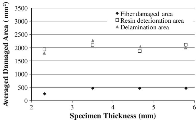
**Fig. 16.** Relationship between damaged area and specimen thickness (condition IV: 4/20  $\mu$ s, 40 kA,  $t = 4.7$  mm)
