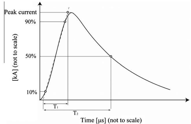
Fig. 5. Impulse waveform definition.
