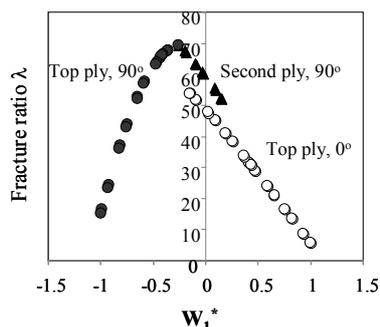
Fig.3 Fracture ratio of all possible cross-ply laminates
