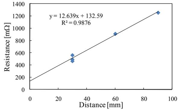
Fig. 7 Resistance values for the various distances for the initial condition
