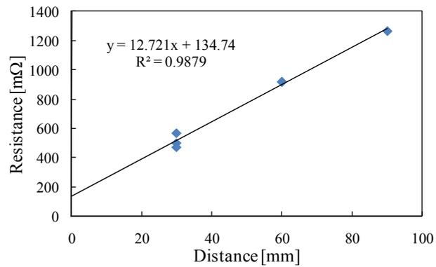
Fig. 8 Resistance values for the various distances after the first cycle loading
