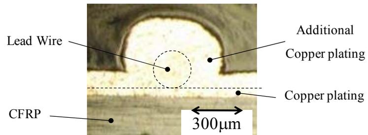
Fig.2 Cross-section view of the new copper plating electrode
