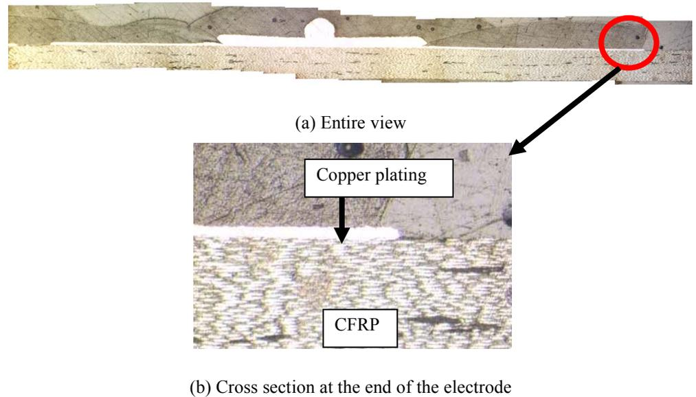
Fig. 15 Cross sectional view of electrode after cyclic loading of  $10^6$  cycles
