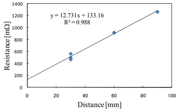
Fig. 10 Resistance values for the various distances after the third cycle loading
