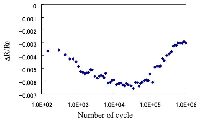
Fig.14 Fraction of electrical resistance change of cyclic loading test of  $[0_4]_T$ .
