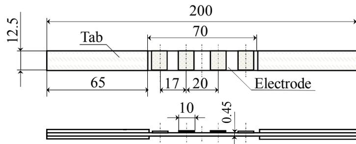
Fig. 6 Specimen configuration of tensile and cyclic loading tests
