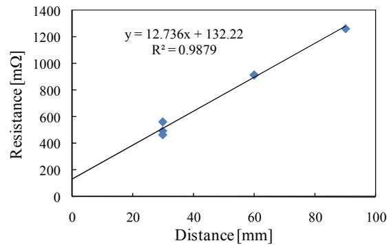
Fig. 11 Resistance values for the various distances after the 100th cycle loading
