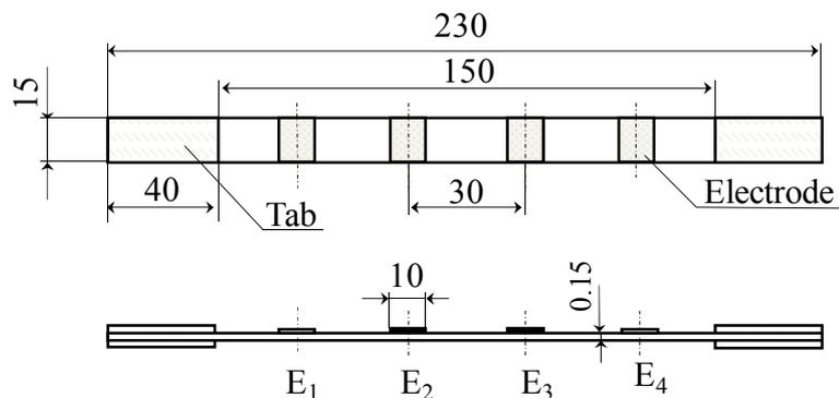
Fig.3 Configuration of a single-ply specimen
