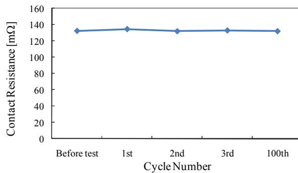
Fig.12 Measured contact resistance after various cyclic loadings
