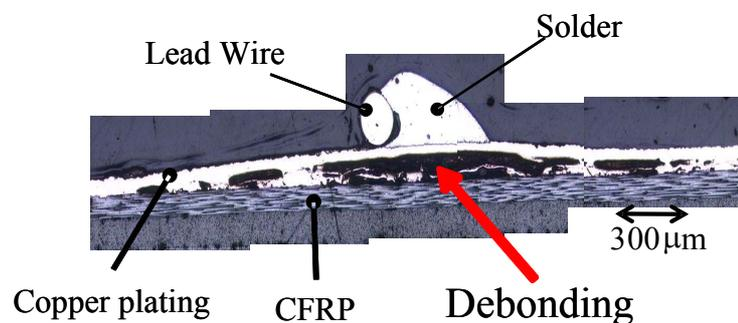
Fig.1 Cross-section of the electrodes made by previous method
