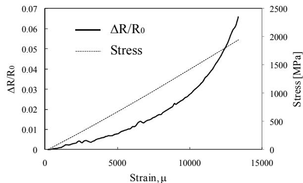
Fig. 13 Fraction of electrical resistance change for the tensile test of  $[0_4]_T$ .
