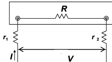
Fig.4 Schematic representation of two-probe method
