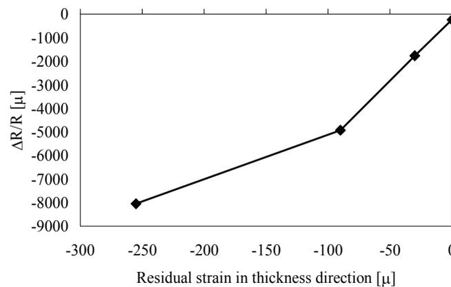
Fig. 4 Measured effect of a dent on the electrical resistance
