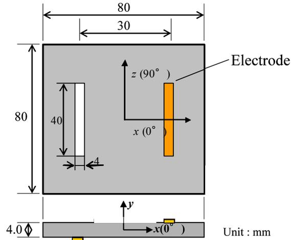
Fig.1 Specimen configuration of a thick CFRP plate
