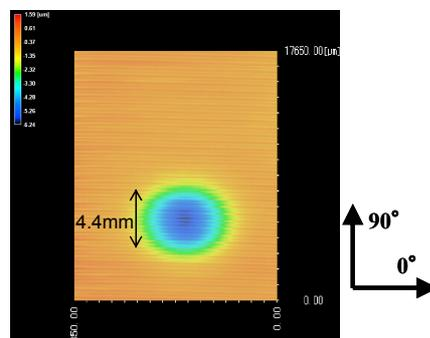
Fig.6 Typical dent configuration measured by using the LASER profilometer
