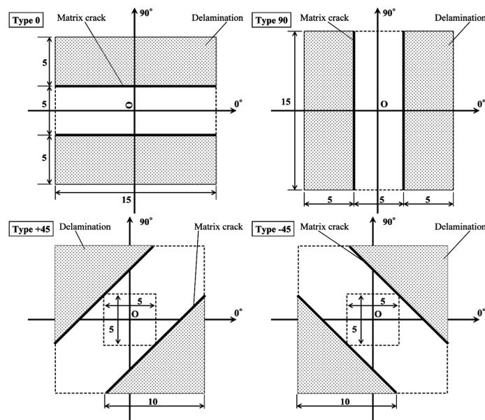
Fig.9 Delamination model used for FEM analyses
