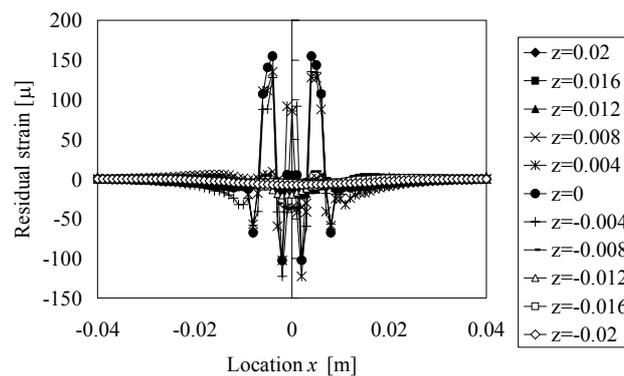
Fig. 12 Residual strain relief of  $x$ -direction strain in each ply
