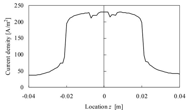
Fig.11 Electric current density in the thickness direction at the middle interlamina
