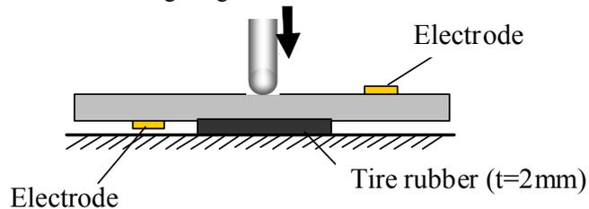
Fig.3 Test method to make a dent without delamination cracks
