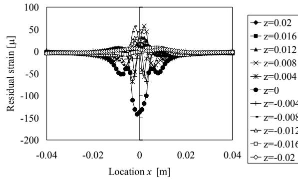
Fig.13 Residual strain relief of  $z$ -direction strain in each ply
