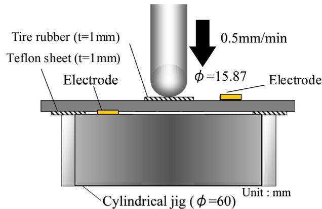
Fig.2 Jig to make delamination crack
