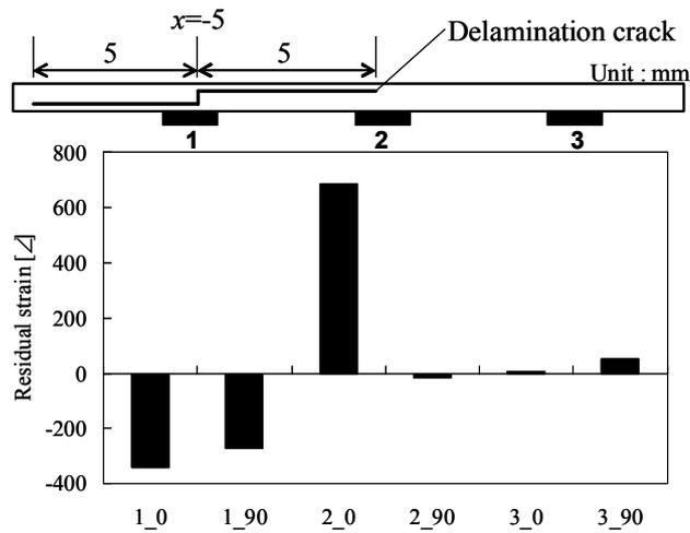
Fig.7 Measured residual strain relief after delamination cracking.
