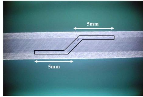
Fig.6 Specimen side surface of delamination cracking.
