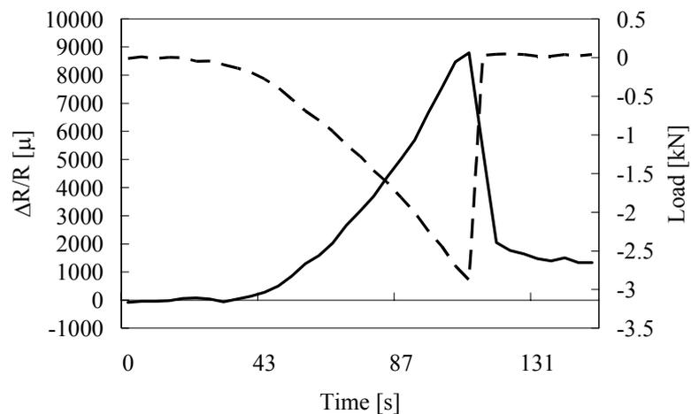
Fig.5 Load-displacement and electrical resistance change-displacement curves.
