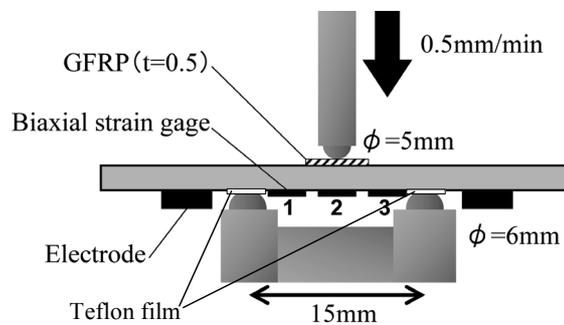
Fig.2 Interlaminar shear test to make a delamination crack.
