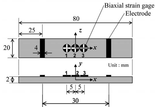
Fig.1 Specimen configuration.
