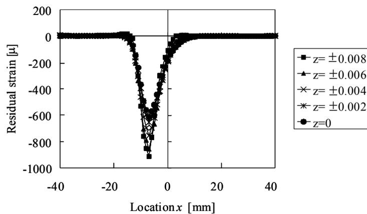
(b) Residual strain relief of y-direction strain.
