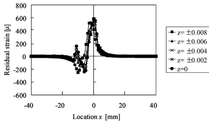
(a) Residual strain relief of x-direction strain
