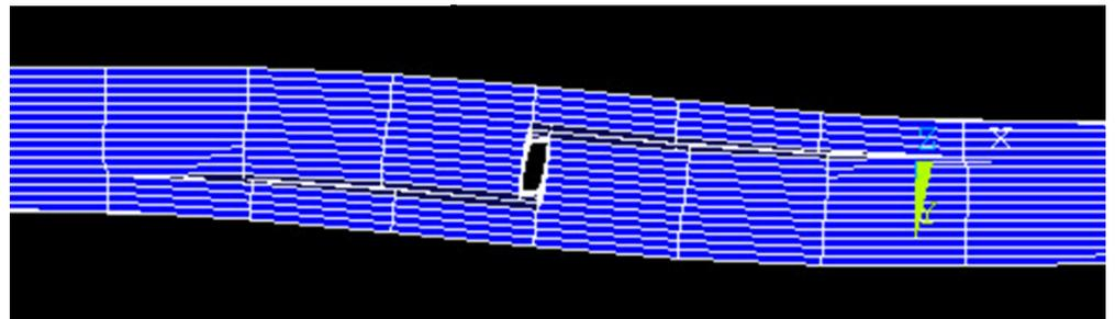
Fig.9 Magnified deformation of FEM result after delamination cracking with consideration of residual strain relief.
