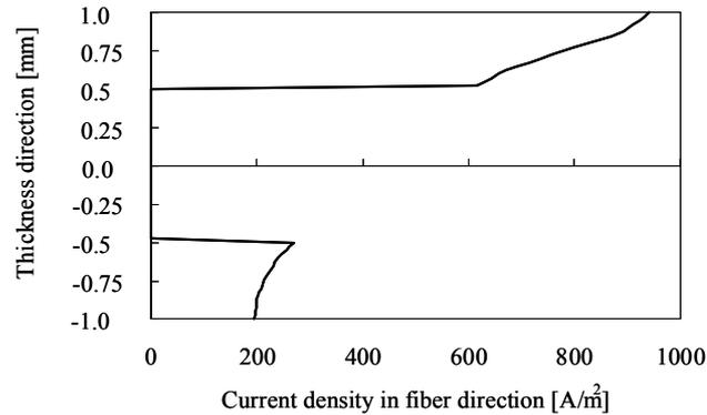
Fig.8 Electric current density (x-direction) distribution by FEM
