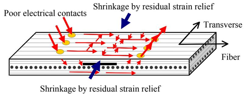
Fig.4 Illustration of piezoresistance effect.
