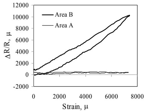
Fig. 14  $\Delta R/R$  due to deformation in the case of simultaneous measurements by the proposed method
