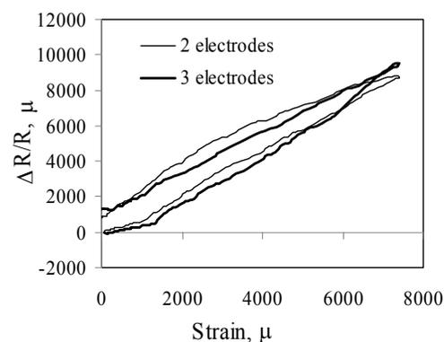
Fig. 12  $\Delta R/R$  due to deformation between electrodes 3 and 5
