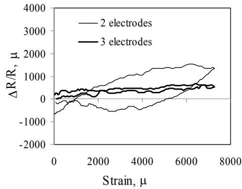
Fig. 13  $\Delta R/R$  due to deformation between electrodes 1 and 3
