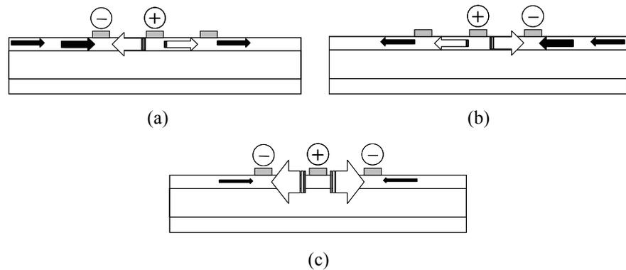
Fig. 4 Electric current density in the surface layer in the cases of (a) the two electrode method using electrodes 1 and 2, (b) the two electrode method using electrodes 2 and 3, and (c) the three electrode method using electrodes 1, 2 and 3
