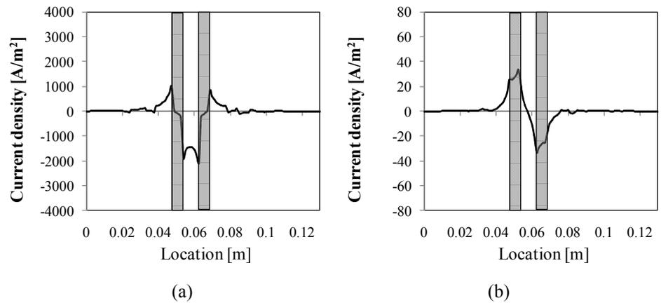
Fig. 7 Current density on the CFRP surface using electrodes 3 and 4 in (a) the longitudinal direction and (b) the thickness direction
