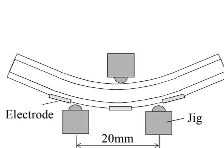
Fig. 10 Inter-laminar shear test
