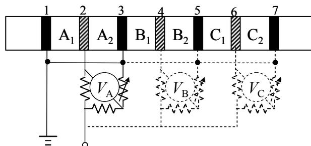
Fig. 3 Three electrode method
