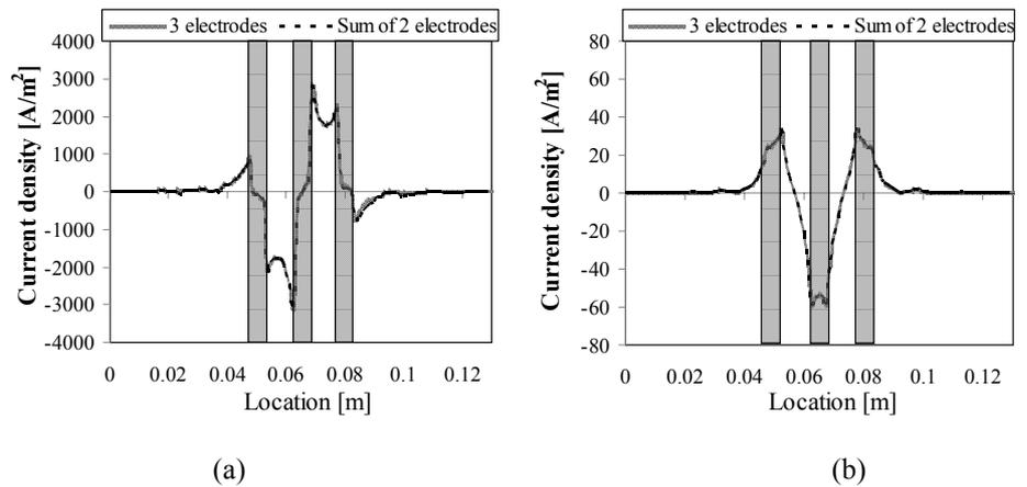
Fig. 8 Current density on the CFRP surface using electrodes 3, 4 and 5 in (a) the longitudinal direction and (b) the thickness direction
