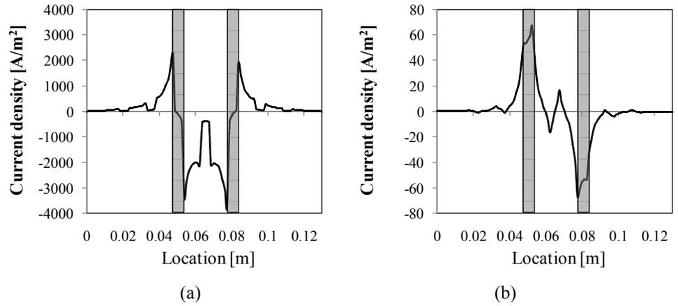
Fig. 6 Current density on the CFRP surface using electrodes 3 and 5 in (a) the longitudinal direction and (b) the thickness direction
