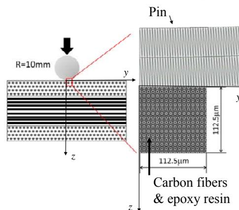
Fig.5 Mesh division of elastic-plastic FEM analysis.
