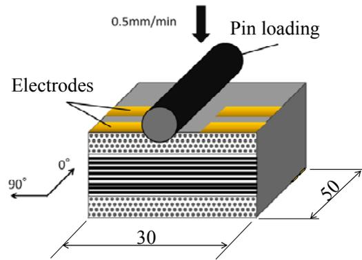
Fig. 4 Configuration of the pin-loading test.
