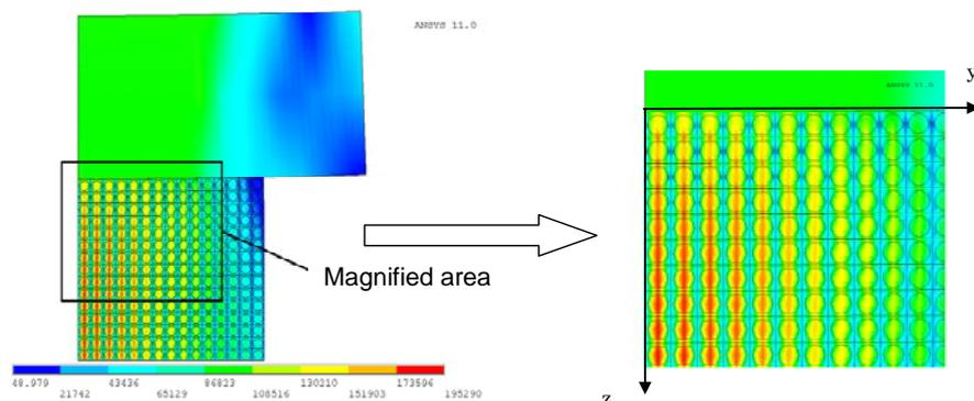
Fig. 14. Equivalent stress distribution obtained using the plane-strain elastic-plastic FEM analysis.
