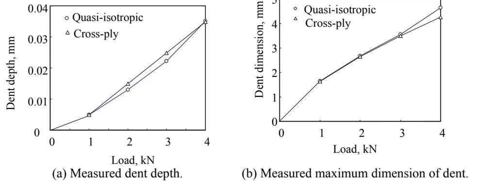
Fig. 7. Measured dent dimensions from the indentation tests.
