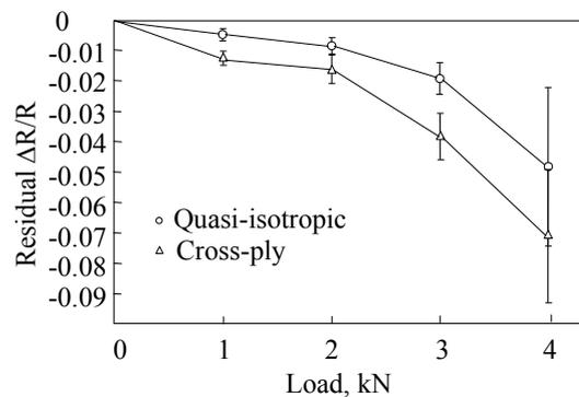
Fig.8 Electrical resistance change ratio of indentation-loading specimen.
