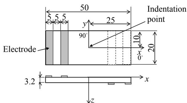
Fig.1 Indentation-loading specimen.
