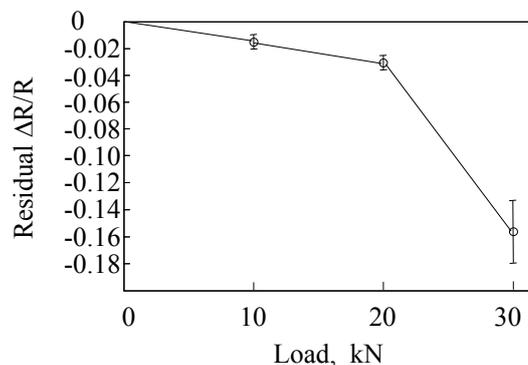
Fig. 11. Electrical resistance change ratio (pin-loading).
