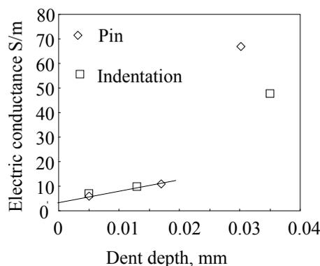
Fig. 15. Estimation results for electric conductance in the thickness direction under the dent area.
