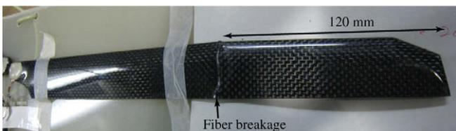
Fig. 12. Damaged blades after three-point bending.
