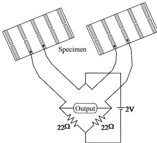
Fig.11. Temperature compensation bridge circuit.
