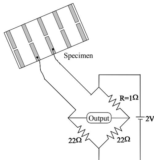
Fig.3. Bridge circuit.
