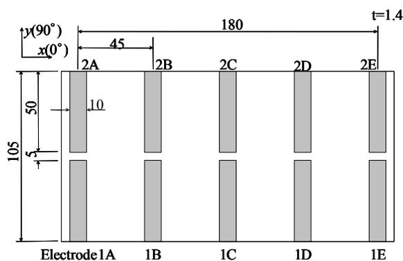
Fig. 1. Specimen configuration.
