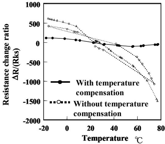
Fig.10. Effect of temperature on resistance change.
