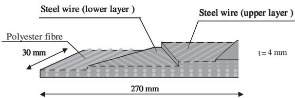
Figure 5. Tyre specimen configuration.
