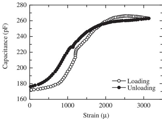
Figure 9. Measured capacitance change during loading and unloading.
