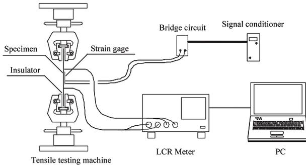
Figure 7. Experimental set-up for capacitance measurement.
