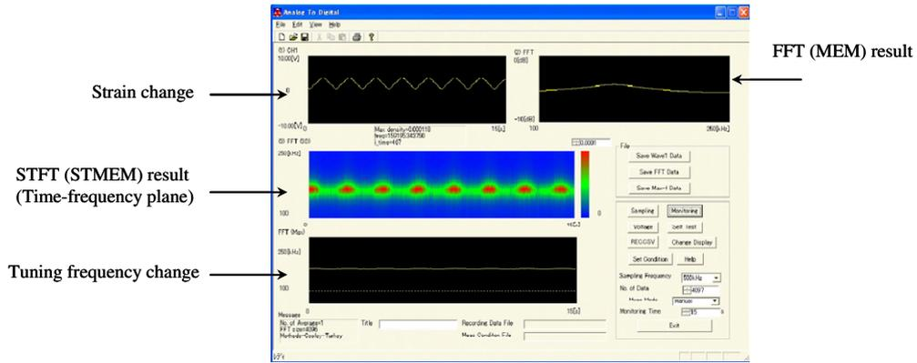
Figure 8. Developed software for spectrum monitoring.
