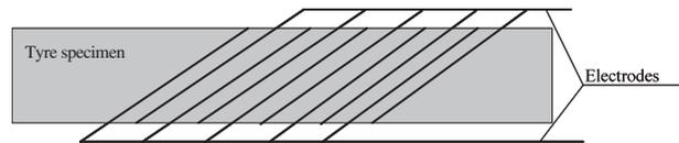
Figure 6. Interdigital electrodes ( $N_d = 10$ ).
