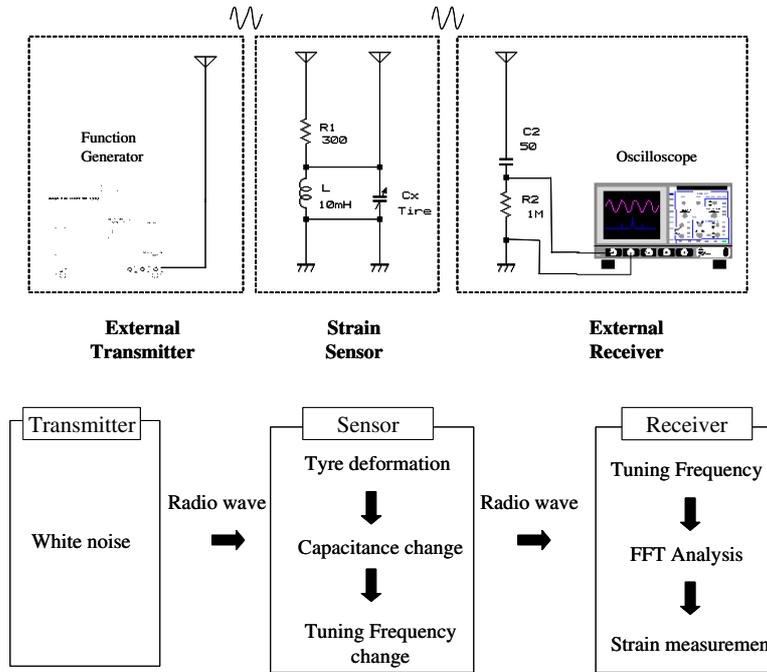
Figure 4. Schematic image of the wireless strain measurement system.
