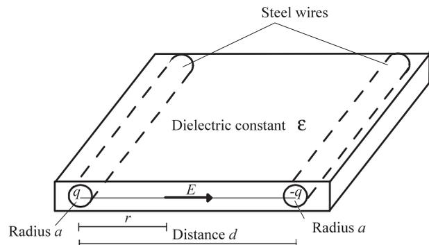
Figure 2. Condenser model of a steel wire belt of a tyre.
