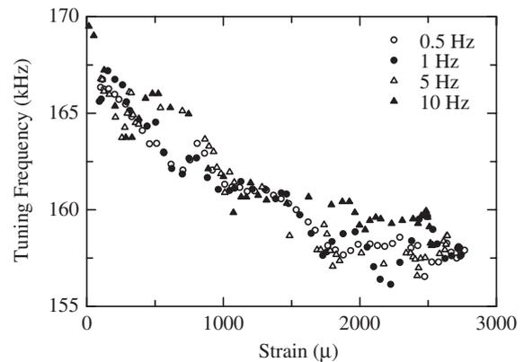
**Figure 14.** Measured relationships between tuning frequency and strain.
