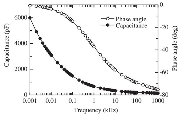
Figure 10. Frequency response of the capacitance and phase angle of the tyre specimen.
