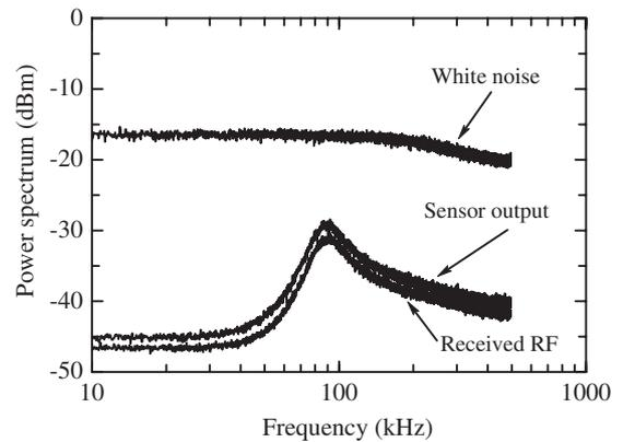
Figure 11. Measured power spectrum of white noise, sensor output, and received RF signal.
