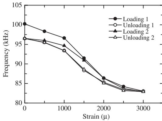
**Figure 12.** Measured relationship between strain and tuning frequency change of the passive wireless sensor.
