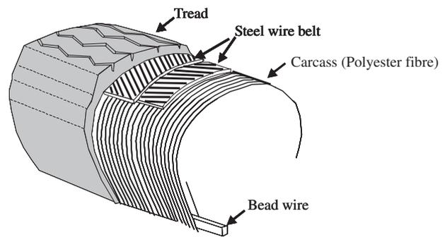
Figure 1. Inner structure of a steel-wire-reinforced radial tyre.
