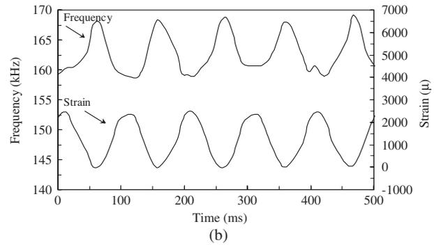
**Figure 13.** Measured tuning frequency change of the passive wireless sensor and strain change. (a) Stroke frequency: 1 Hz. (b) Stroke frequency: 10 Hz.
