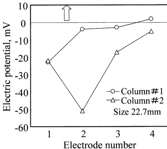
Fig. 8. Measured electric potential distribution at each electrode when the delamination exists at column #2 and line #2 ( $x = 64.9$ ,  $y = 82.9$ ).
