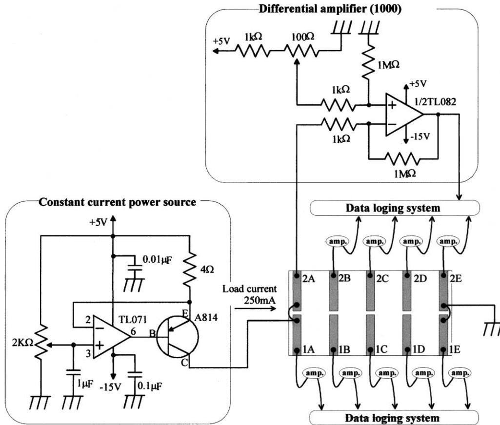
Fig. 5. Electric circuit used for voltage change method.
