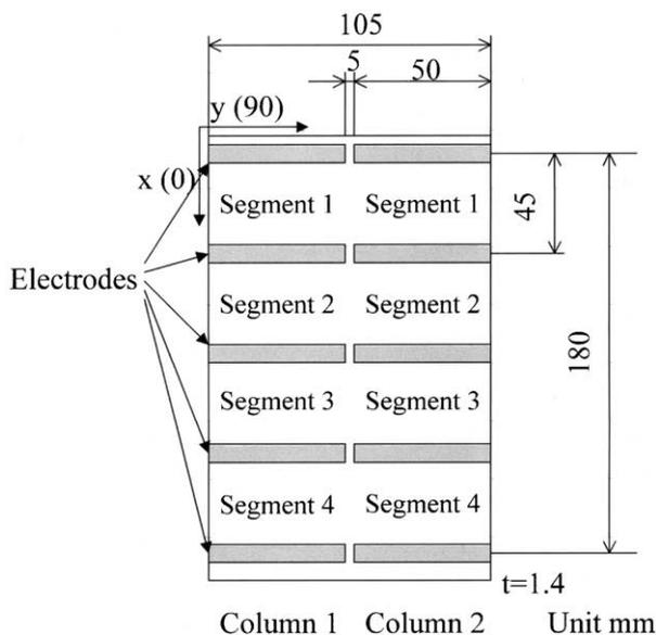
Fig. 4. Specimen configuration.
