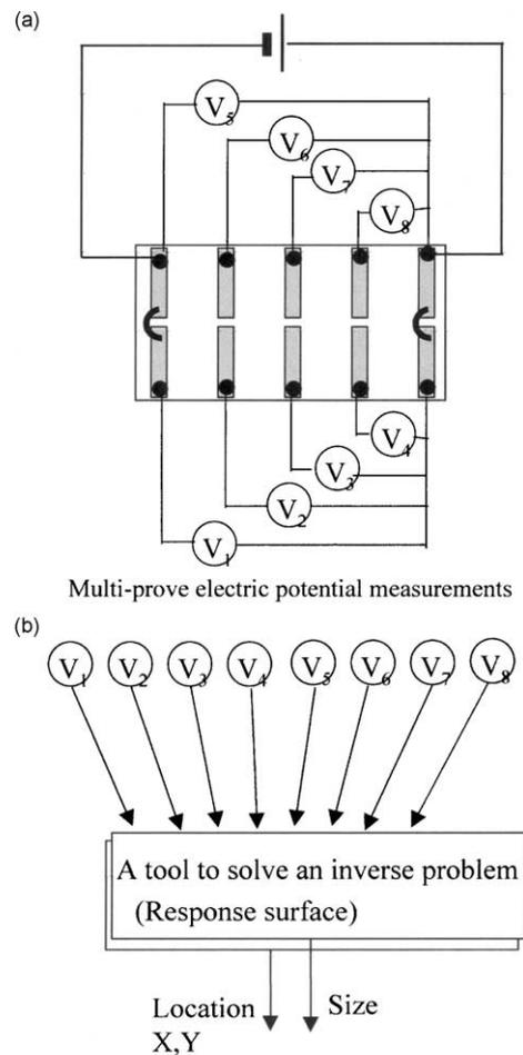
Fig. 3. Schematic representation of delamination identification method using multi-probe electric potential change method with response surfaces.
