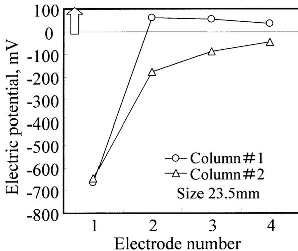
Fig. 7. Measured electric potential distribution at each electrode when the delamination exists at column #1 and line #1 ( $x = 24.1$ ,  $y = 21.2$ ).
