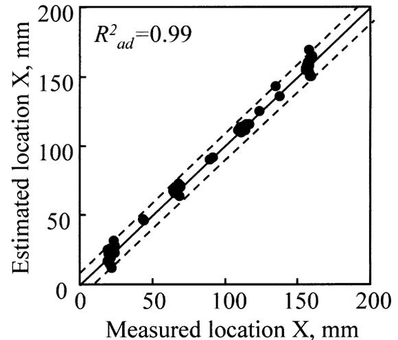
Fig. 9. Estimated delamination location of X direction with error band of 10 mm.
