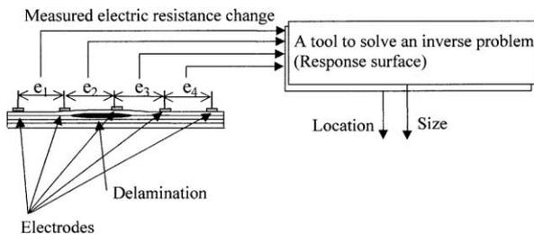
Fig. 2. Schematic representation of delamination identification method using electric resistance change method with response surfaces.
