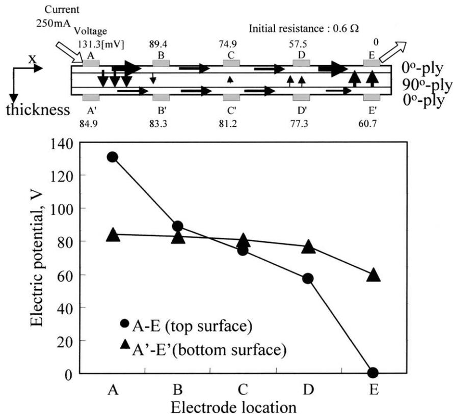
Fig. 6. Electric potential distribution and schema of electric current.
