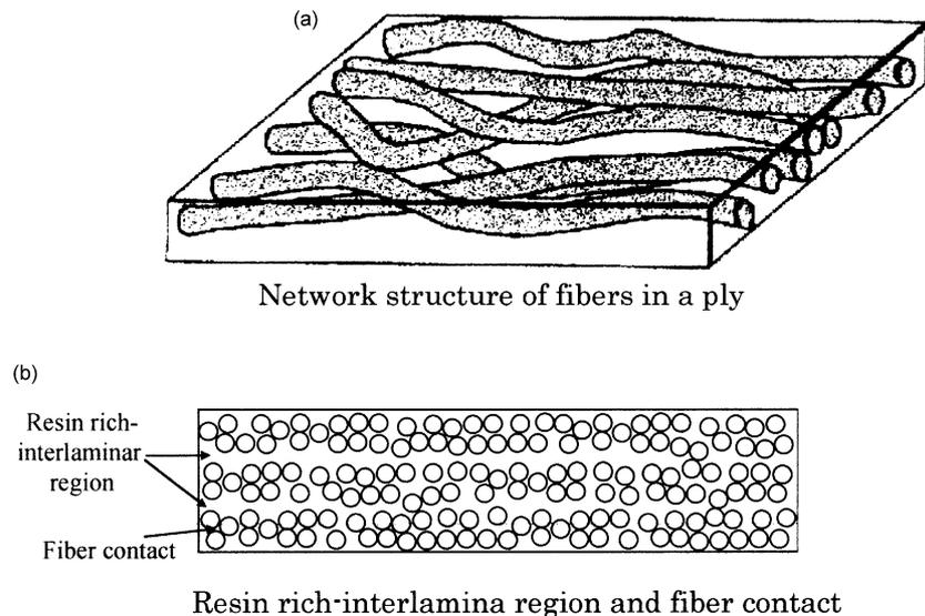
Fig. 1. Schema of practical structure of graphite/epoxy composite.
