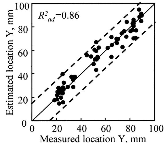
Fig. 10. Estimated delamination location of Y direction with error band of 15 mm.
