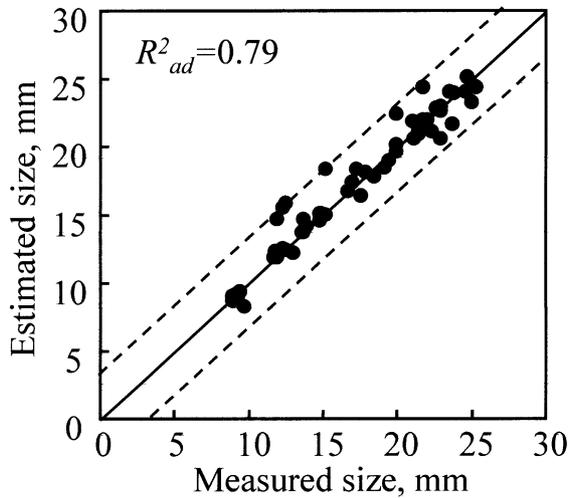
Fig. 11. Estimated delamination size error band of 3 mm.
