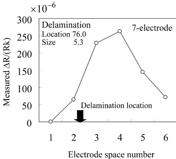
Fig. 10. Measured electric resistance of type E specimen.
