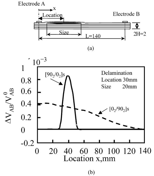
Fig. 3. Effect of stacking sequences for electric voltage change distribution after delamination creation. (a) FEM analysis model; (b) electric voltage change distribution on specimen surface by FEM analysis of cross-ply laminates.
