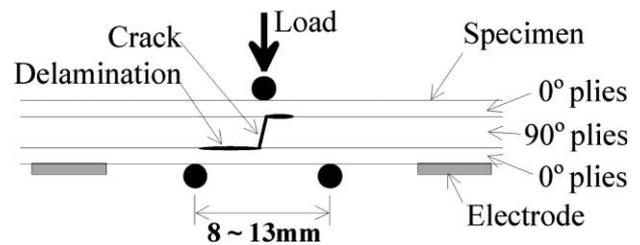
Fig. 7. Method for delamination creation.
