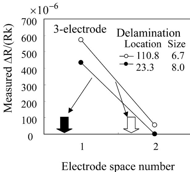
Fig. 9. Measured electric resistance of type A specimen; two results of specimens that have different delamination but have similar results.
