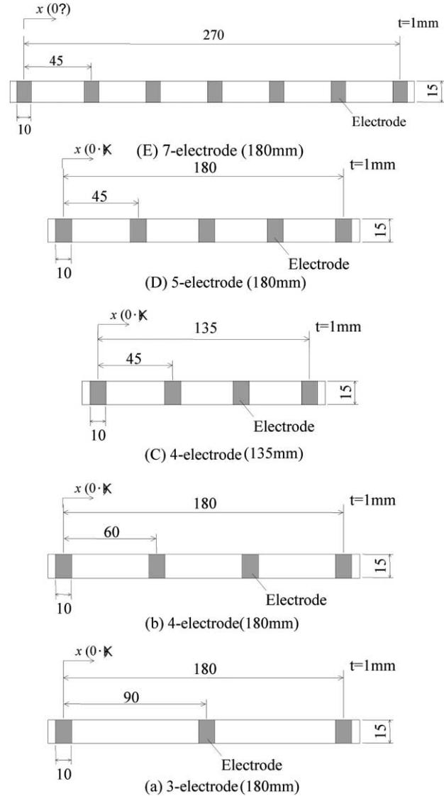
Fig. 5. Specimen configurations.
