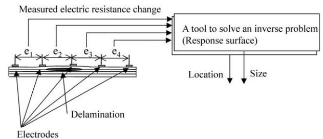
Fig. 4. Schematic representation of delamination identification method using electric resistance change method with response surfaces.
