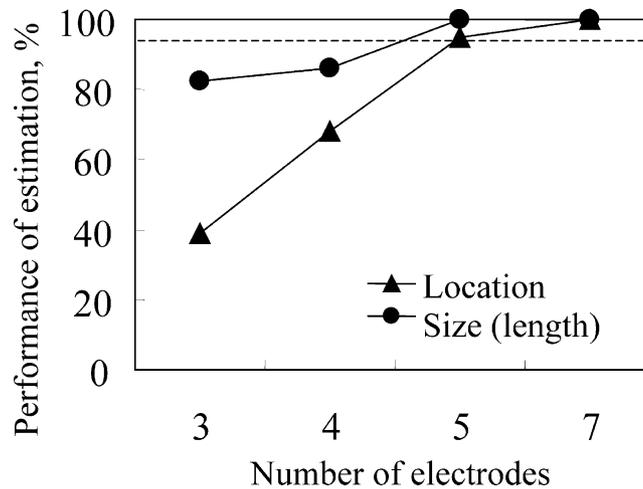
Fig. 13. Effect of the number of electrodes on the practical performance of estimations of location and size.
