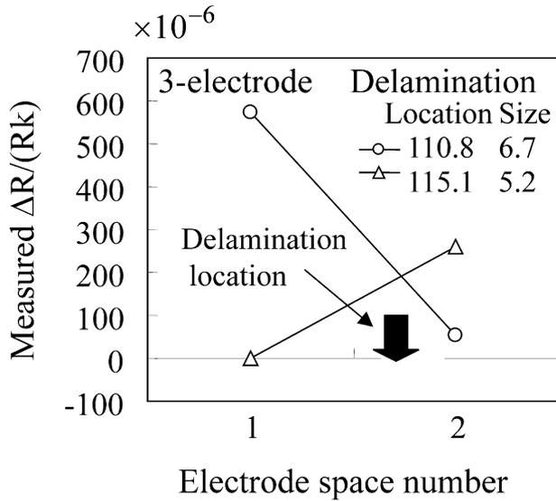
Fig. 8. Measured electric resistance of type A specimen; two results of specimens that have similar delamination with each other.
