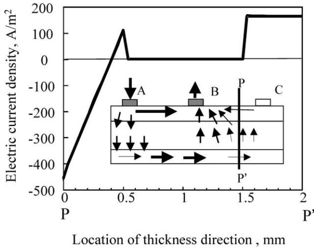
Fig. 2. FEM analysis of electric current density at the cross section P–P' when the electric current is charged between A and B (A:30 mA, B:0 V);  $\sigma_{90}/\sigma_0 = 10^{-3}$  and  $\sigma_t/\sigma_0 = 10^{-4}$  [11].
