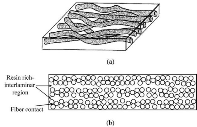
Fig. 1. Schema of practical structure of graphite/epoxy composite. (a) Network structures of fibers in a ply; (b) resin rich-interlamina region and fiber contact.
