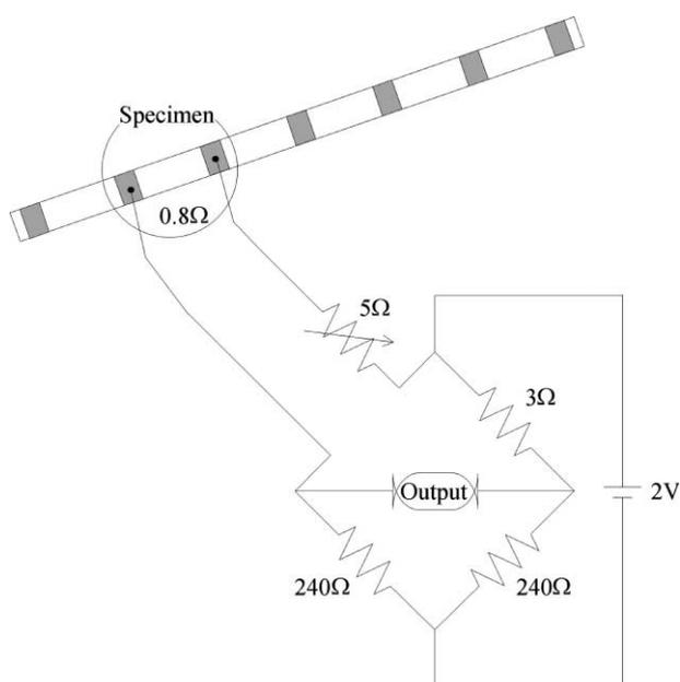
Fig. 6. Electric resistance bridge circuit employed in the present study.
