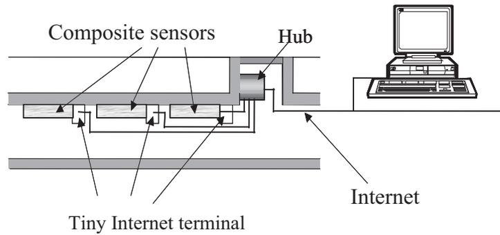
**Figure 1** Schematic image of monitoring system.
