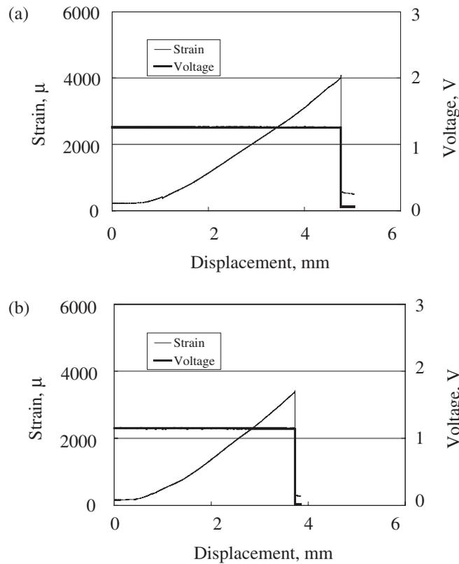
**Figure 9** Experimental results of 4-point bending test: (a) Number of surface plies is 1; (b) number of surface plies is 2; (c) number of surface plies is 3; and (d) number of surface plies is 4.
