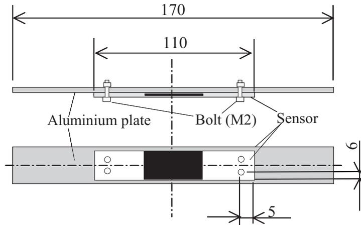
Figure 7 Composite sensor with aluminium plate for 4-point bending test.
