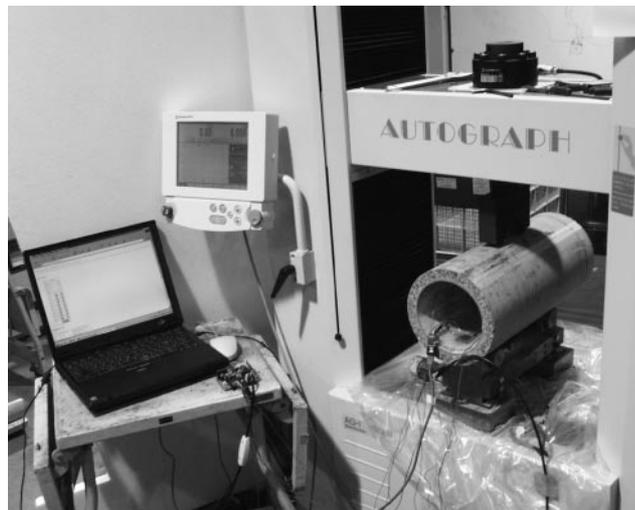
**Figure 14** Experimental setup of demonstration test of fracture monitoring of sewer pipe.
