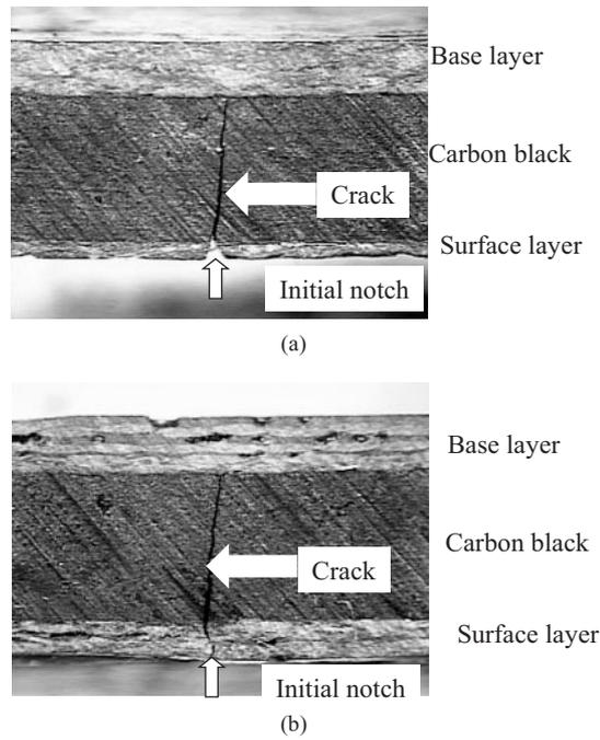
Figure 10 Cracks in composite sensors: (a) Number of surface plies is 1; (b) number of surface plies is 2; (c) number of surface plies is 3; (d) number of surface plies is 4.
