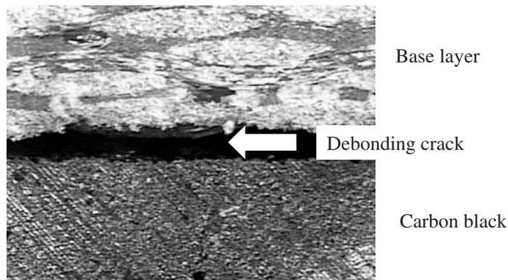
**Figure 12** Debonding between carbon sheet and glass composites.
