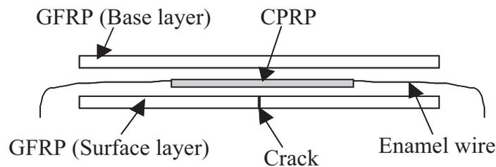
**Figure 4** Schematic image of a fracture sensor.
