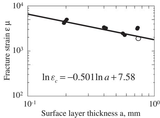
Figure 11 Relationship between fracture strain and surface thickness.
