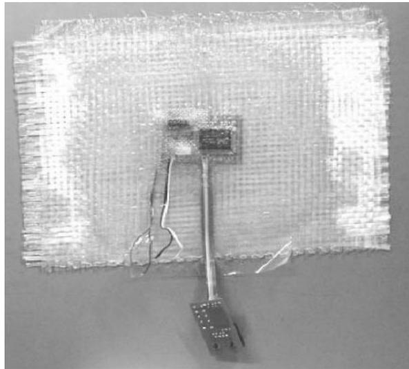
**Figure 5** Embedded tiny terminal in glass–epoxy composites.
