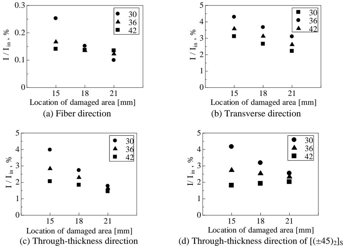
Fig.4 Electrical current ratio through different internal cross sections that correspond to delamination, fiber breaking and matrix cracking
