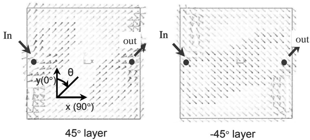
Fig.2 Vector diagram of electrical current density in 45° and -45° layer of [45/0/-45/90]<sub>s</sub> laminate
