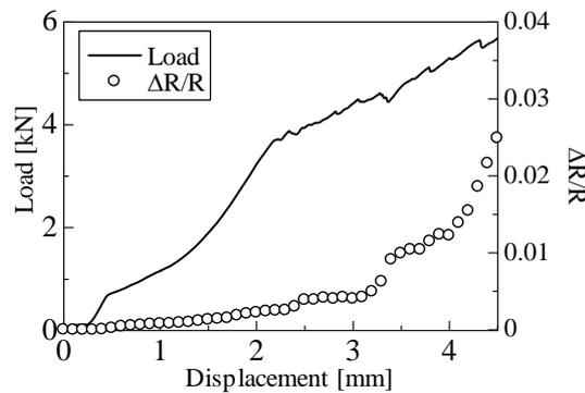
Fig.6 Experimental electrical resistance change by bearing failure [30]
