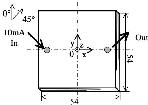
Fig.1 Analytical model of CFRP plate for the electrical resistance change method
