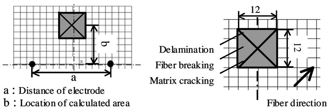
Fig.3 Internal cross-sections to calculate electrical current ratio
