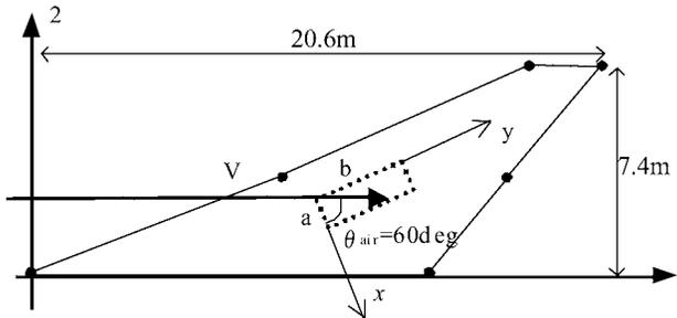
**Figure 12.** Coordinates of SST wing and supersonic flow.
