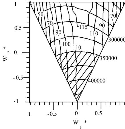
**Figure 11.** Contour plot of response surface of flutter speed limit with buckling load ratio  $\varphi = 30^\circ$   $a/b = 1$ .
