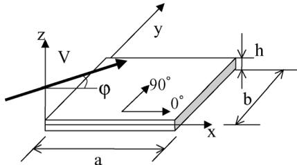
**Figure 1.** Coordinates of the laminate and supersonic flow.
