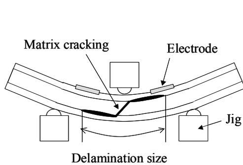
Fig. 4 Schema of delamination
