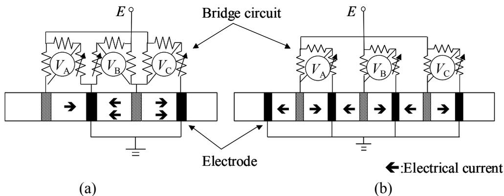
Fig.1 Measurement method of multiple electrical resistance changes
