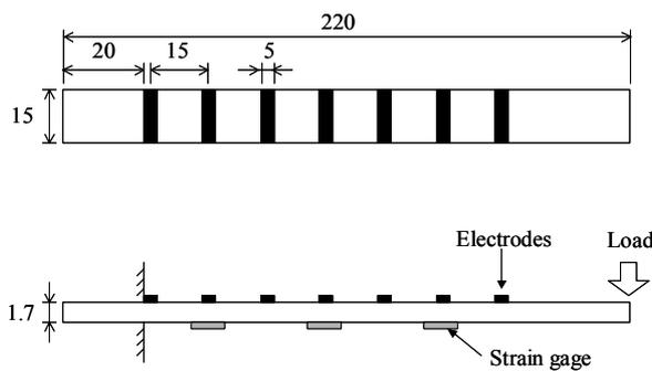
Fig.2 Specimen configuration
