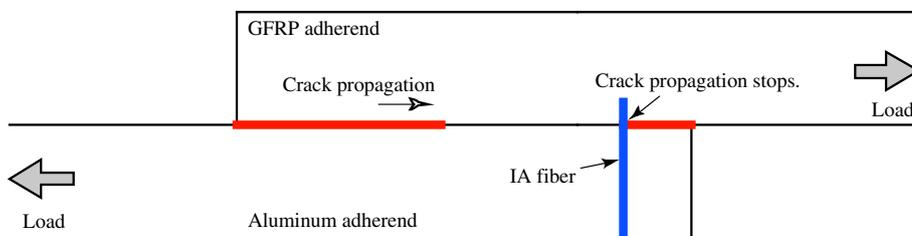
Fig. 11. Side view of the IAF joint in Phase IV: the crack previously formed at the aluminum edge stops at the IAF point while another crack propagates from the GFRP edge.
