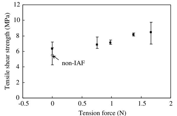
Fig. 15. Effect of tension force of the IA fiber on the tensile shear strength of IAF joints: IAF joint (square symbol); non-IAF joint (circle symbol).
