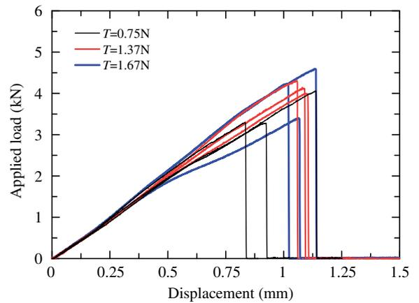
Fig. 14. Load–displacement curves of the IAF joint varying the tension force of the IA fiber: 0.75 N, 1.37 N, and 1.67 N.
