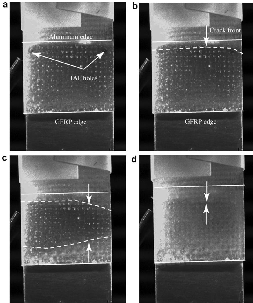
Fig. 10. Crack propagation of the IA joint during tensile shear tests: (a) Phase I; (b) Phases II and III; (c) Phase IV; (d) the adhesive joint failure at B4. The solid line indicates the edges of aluminum and GFRP adherends; the dashed lines are the crack fronts.
