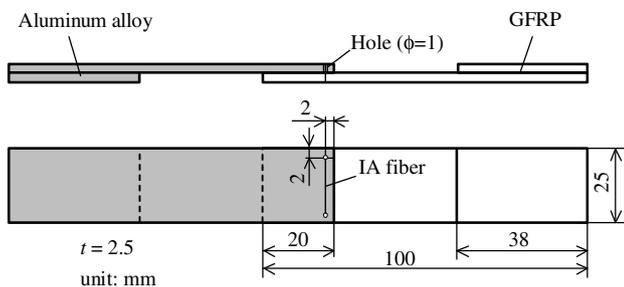
Fig. 3. Specimen configuration of the IAF joint between GFRP and aluminum.
