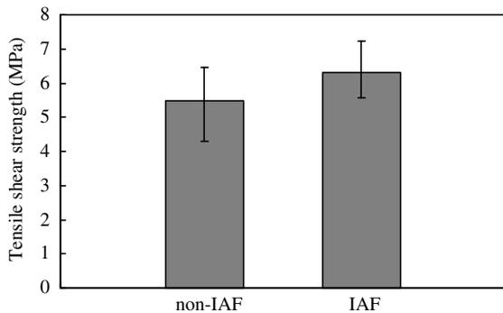
Fig. 13. Average static tensile shear strengths of aluminum/GFRP non-IAF and IAF joints.
