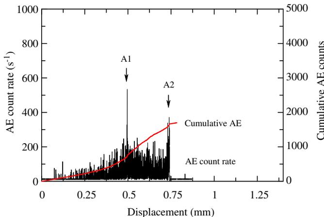
Fig. 8. Acoustic emission (AE) count rate and cumulative AE counts for non-IAF joints during static tensile–shear tests. A1 and A2 correspond to the same numbers in Fig. 7.
