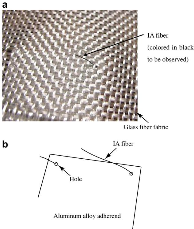
Fig. 2. Stacking process of the IAF joint using plain woven fabric GFRP. The IA fibers are inserted between the glass fiber warp and weft bundles without damaging fibers: (a) photograph; (b) illustration.
