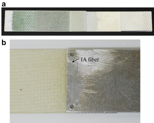
Fig. 5. Photograph of the aluminum/GFRP IAF joint specimen: (a) specimen overview (GFRP surface); (b) zoomed at the IAF (aluminum surface).
