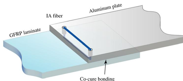
Fig. 1. Schematic illustration of the Inter-Adherend-Fiber joint between aluminum and GFRP laminate. The IA fiber penetrates into the GFRP and holes in the metal adherend, and unites both adherends with co-cure bonding.
