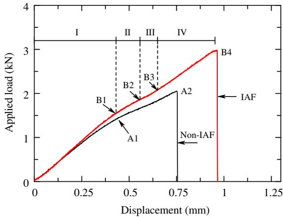
Fig. 7. Applied load and displacement diagram of aluminum/GFRP non-IAF and IAF joints. Adhesive crack and adhesive joint failure occur at A1 and A2 in the non-IAF joint, respectively. For the IAF joint, a crack occurs at the aluminum edge at B1; and propagates to the position of the IAF; the crack propagation stops at B2 until B3; another crack occurs at the GFRP edge at B3 and progresses to the aluminum edge; and finally the IAF joint breaks at B4.
