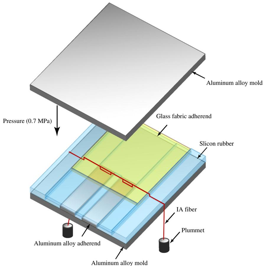
Fig. 4. Illustration of co-curing process of IAF joint specimens.
