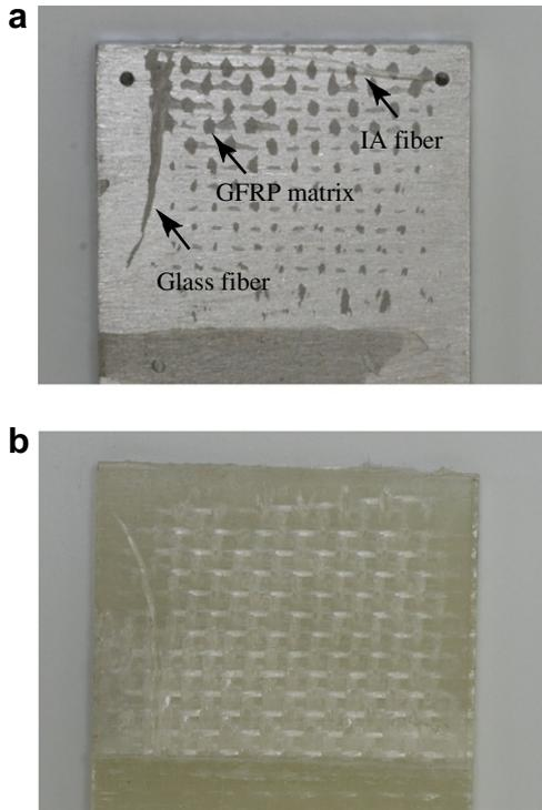
Fig. 12. Failure surfaces of the aluminum/GFRP IAF joint after static tensile shear tests: (a) aluminum adherend; (b) GFRP adherend.
