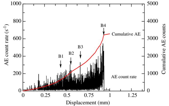
Fig. 9. Acoustic emission (AE) count rate and cumulative AE counts for IAF joints during static tensile–shear tests. B1, B2, B3 and B4 correspond to the same numbers in Fig. 7.
