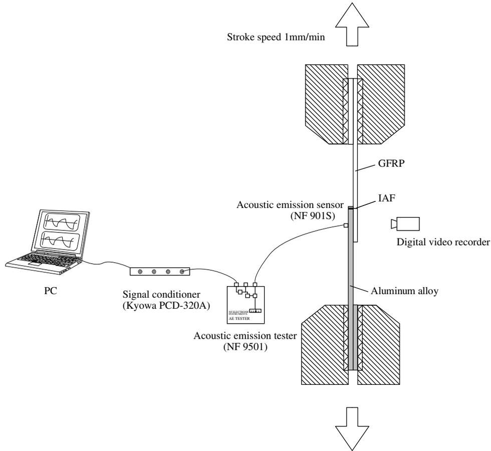
Fig. 6. Experimental setup of tensile lap-shear tests.
