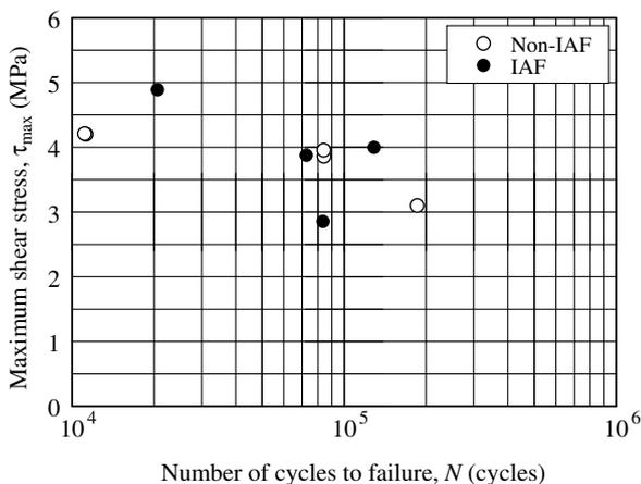
Fig. 16. Maximum shear stress and number of cycles to failure for the aluminum/GFRP non-IAF joint (open circles) and IAF joints (solid circles). The stress ratio  $R$  is 0.1.
