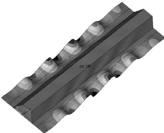
Fig. 8. Buckling mode shape of quasi-isotropic laminates. Skin:  $[45/0/90/-45/90/-45/45/0]_S$ , stiffener:  $[45/0/90/-45/90/-45/45/0]_S$ , buckling load ratio:  $\lambda = 4.253$  (FEM).
