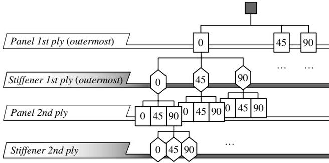
Fig. 1. Alternating stacking sequence optimization process of stiffened panel.
