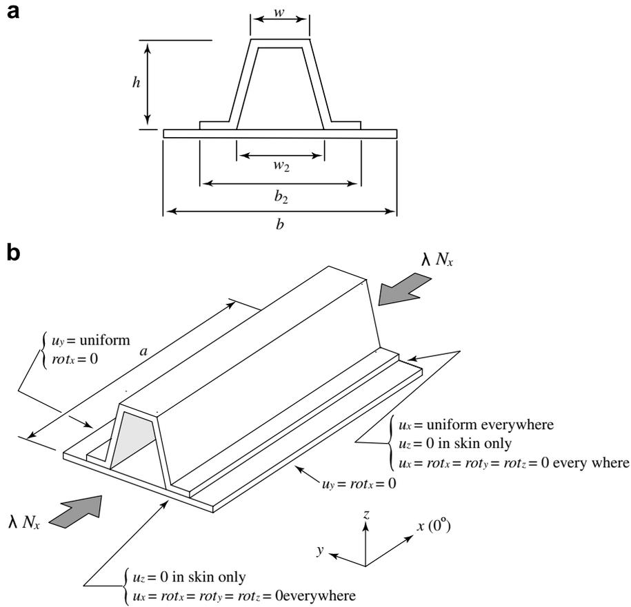
Fig. 5. Analysis model of hat-stiffened panel. (a) Cross section geometry of hat-stiffened panel. (b) The whole view of analysis model.
