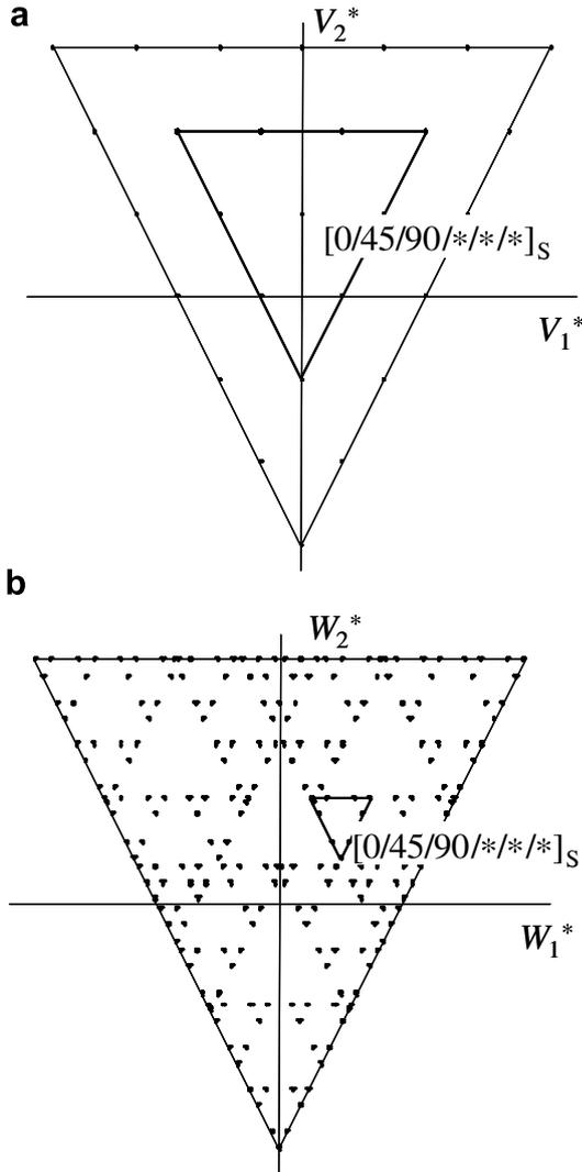
Fig. 2. Fractal pattern drawn by plotting all feasible laminates of 12 plies ( $N = 6$ ): (a) in-plane lamination parameter coordinates, (b) out-of-plane lamination parameter coordinates.
