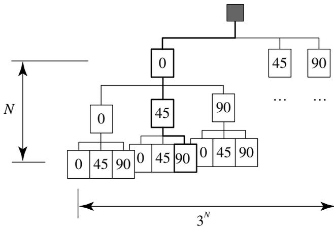
Fig. 3. Tree structure of a stacking sequence.
