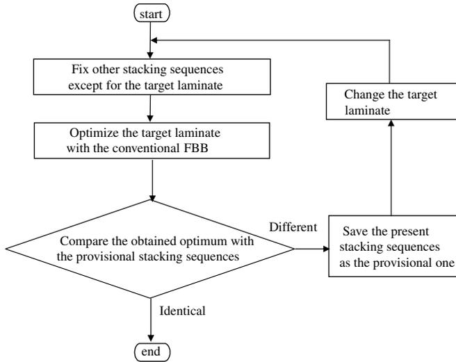
Fig. 4. Flow chart of the new alternating FBB method.
