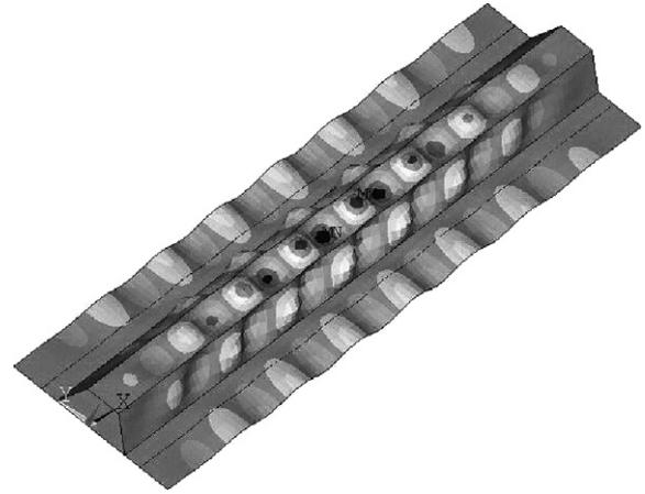
Fig. 9. Buckling mode shape of the true optimal laminates. Skin:  $[(45/-45)_4]_S$ , stiffener:  $[(45/-45)_2/0/90]_S$ , buckling load ratio:  $\lambda = 8.816$  (FEM).
