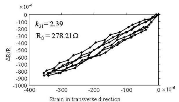
Fig. 3. Measured electrical resistance change in fibre-direction loading of transverse-direction current path.
