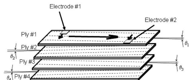
Fig. 8. Misaligned ply model of the unidirectional laminate and electric current path.
