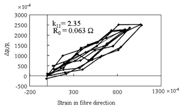
Fig. 2. Measured electrical resistance change in fibre-direction loading of fibre-direction current path.
