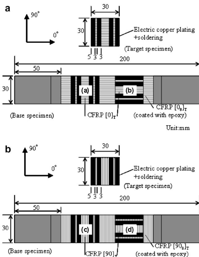
Fig. 1. Specimen configuration. (a) Unidirectional fibre-direction loading and (b) unidirectional transverse-direction loading.
