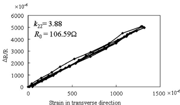
Fig. 5. Measured electrical resistance change in transverse-direction loading of transverse-direction current path.
