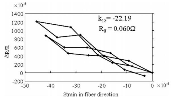
Fig. 6. Measured electrical resistance change in transverse-direction loading of fibre-direction current path.
