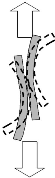
Fig. 4. Fibre-contact separation model to explain positive piezoresistivity in the transverse direction.
