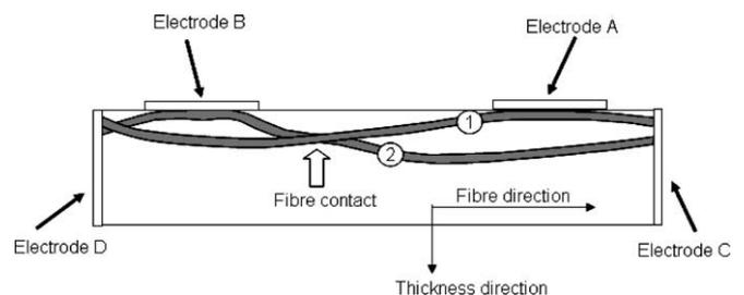
Fig. 7. Actual fibre undulation in a ply and effect of location of electrodes.
